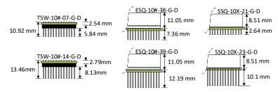
Note: TXS PCB is denoted by the green line. PCB thickness: 1.00mm
