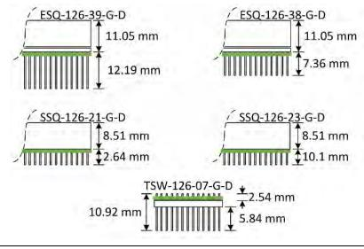
Note: The board location with respect to the connector is marked by the green line in the drawing above (the line represents the PCB).
