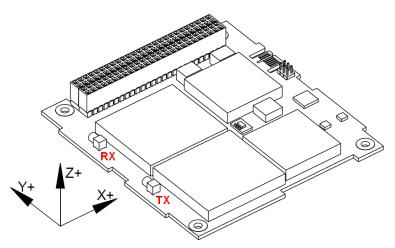
UHF Transmitter (TX) Connector Mounting position and orientation (type is MMCX male)
