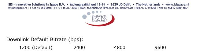
Default data rate of the transmitter at power-up. The data rate can be changed on command after start-up.
