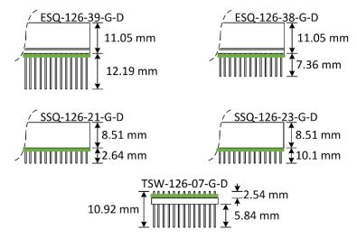
Note: The board location with respect to the connector is marked by the green line in the drawing above (the line represents the PCB).. The iMTQv2 board is 1.7mm thick.
